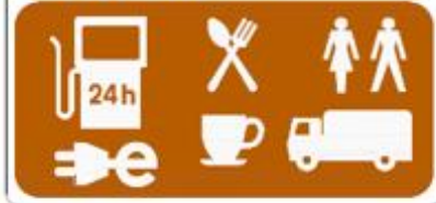
Service Station with HCV Parking on Single Carriageway Network: Advance Information Sign
