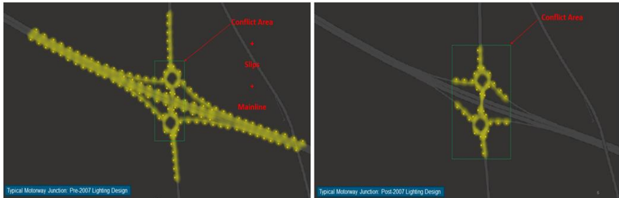
Figure 1 – Typical Large Footprint (Pre-2007) and Small Footprint (Post-2007) junction lighting designs.
